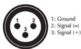
DMX-input XLR mounting-plug:
